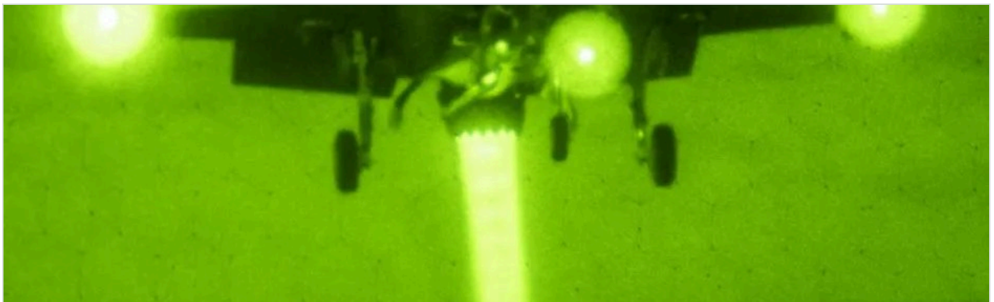
The exhaust jet of an F-35B in vertical landing strikes the ground, at 926 degrees per the reference standard.
